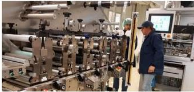
Fig.2 Electrochromic devices can be printed in sheet-to-sheet or roll-to-roll. Ynvisible Production R2R line in Linköping, Sweden.
