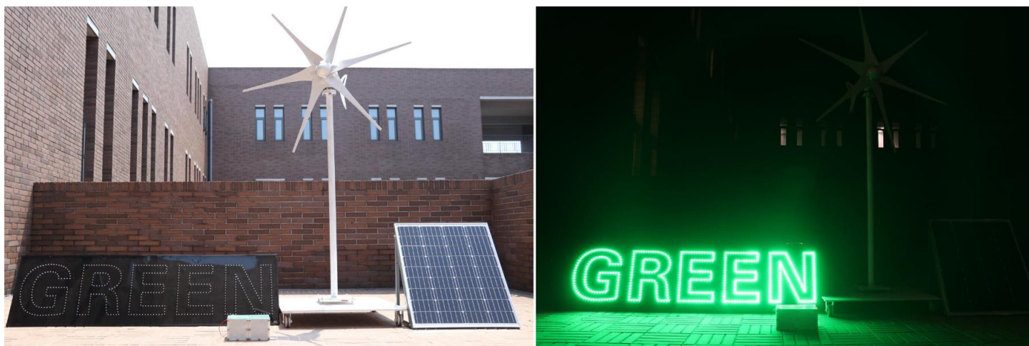
Demonstration of a renewable energy storage system. Photos of the researchers' demonstration of a renewable energy storage system based on a DZMB pack (in the middle of the photo) integrated with solar photovoltaic (PV) modules and a wind-driven generator through a controller. The controller was also connected to a light-emitting diode (LED) panel, serving as the electrical load.
